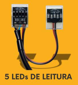
Dynapar's seed sensor is suitable for all types of seeds, regardless of size, shape and seed rate. With 5 readout LEDs, the SSBR accurately counts the seed population during planting, from larger seeds such as corn to small seeds such as sorghum, among others, providing confidence in your planting system and optimizing your productivity.
