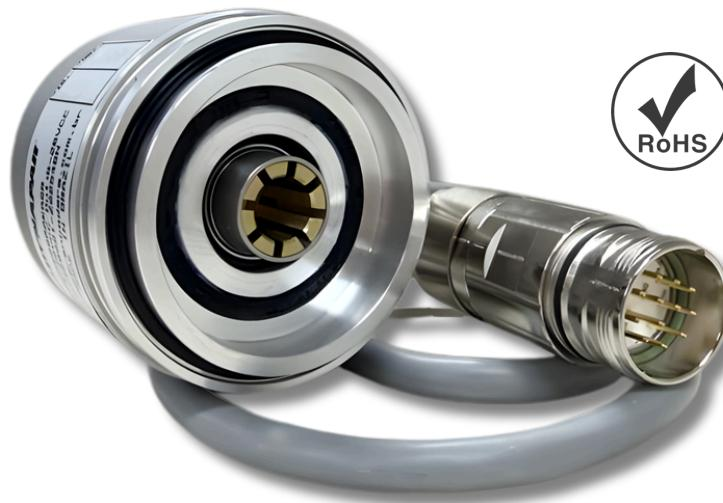
The B58N was developed for the ceramic segment. With a resolution of 1 to 10,000 PPR, HTL output, and A, B, and Z signals, it delivers precision and reliability in a compact 58 mm format and IP67 protection (cover and shaft). Available with cable output or side connector, it easily adapts to different machine configurations.
