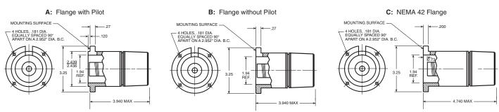
Mating shaft lengths: Typically: 0.5" max. available into the coupling as measured from the A/B mounting surface. 1.3" max. available into the coupling as measured from the C mounting surface.
