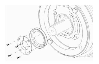
1) Slide the magnetic wheel onto the shaft; align the adapter front surface with housing groove surface.
