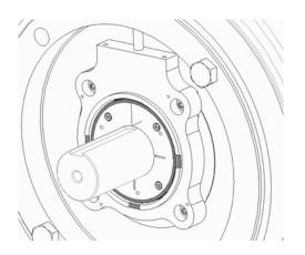
2) Tighten the screws to a nominal of 2.24 N-m.
