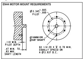
STEP 1: Please reference the below diagram titled "EN 44 Motor Mount Requirements" to ensure that a correct mounting interface is provided for the mechanical installation of this encoder. The EN44 has a 0.110 inch piloted face that is concentric with the Flex Coupling. Be sure to create a concentric pilot with the six 1/4-20 inch threaded holes on customer equipment as shown in the diagram.
