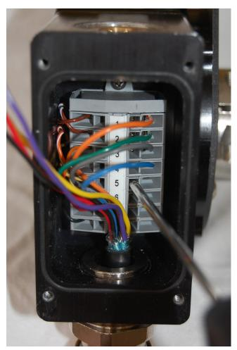
**Step 3:** Wire to terminal block using pin assignment on this page or on the inside of terminal box cover. Carefully press a 1/8" flat blade screw-driver into the inboard hole to open terminal. Insert wire completely and remove screwdriver.
