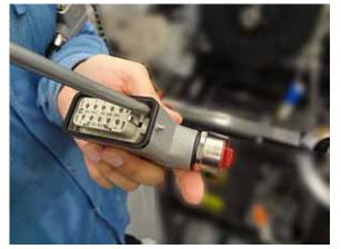
10.0 Pull the mating connector out and complete wiring per electrical connections table
