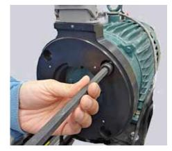
5.0 Slide Clamp wheel on to the shaft
