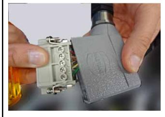
11.0 Latch mating connector to the housing. Installation is complete.
