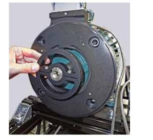
6.0 Position the wheel such that its front surface is flush with housing groove surface.
