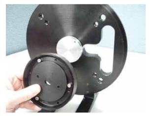
Orient the Shaft adapter to end of the motor. The fit should be snug, but smooth.
