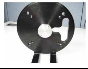
The ST8 Magnetic wheel assembly comes in two versions. "Through Shaft" and "End of Shaft". The Through Shaft version allows the motor shaft to completely transit "through" the center of the magnetic wheel. The wheel is somewhat like a large collar around the shaft. The End of Shaft (EOS) adapters "caps" over the machined end of the motor shaft. This style of shaft mounting is common on larger DC motors.
