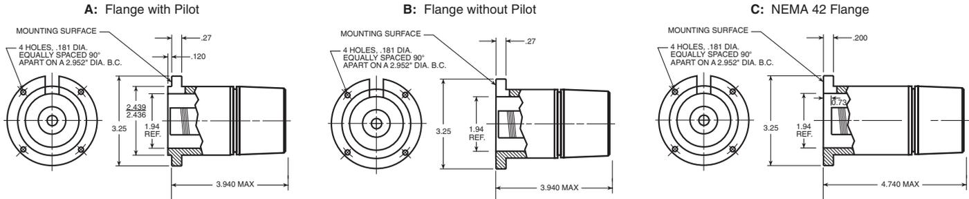
**Mating shaft lengths:** Typically: 0.5" max. available into the coupling as measured from the A/B mounting surface.
